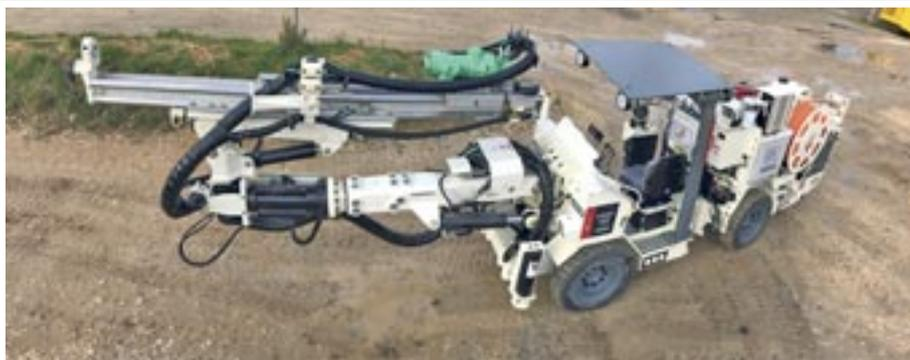
*Aramine's diesel-electric hybrid miniDriller DM901 HDE drill rig uses the diesel engine for tramping and electric motor for drilling*
