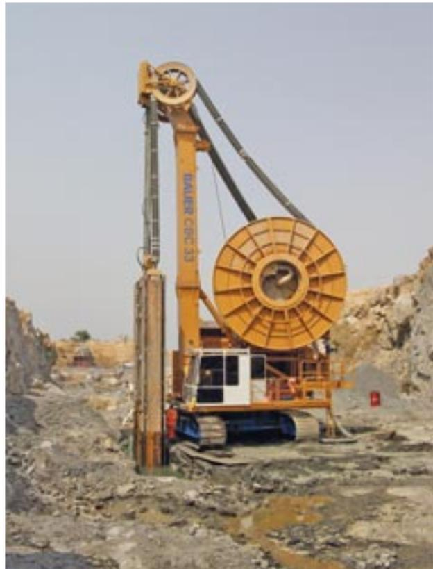
*Looking to mine dykes for kimberlites to a greater depth, Koidu Limited and Bauer Technologies, in 2010, agreed to trial the BC 33 cutter at its kimberlite mining leases in Sierra Leone*
