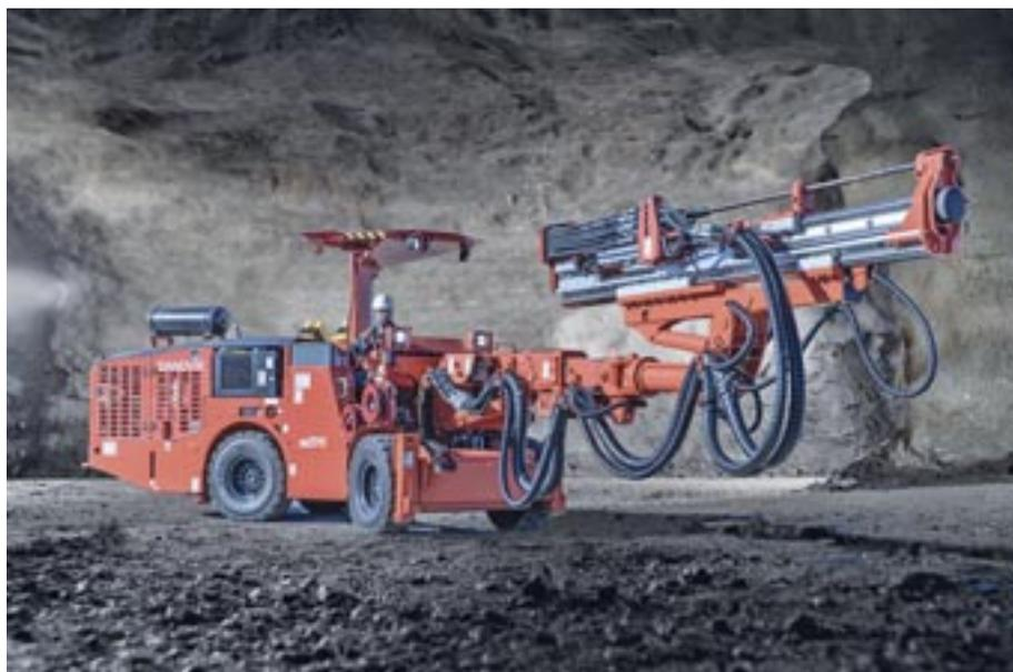
cross section of 2.7 m x 2.7 m. The versatile boom delivers large coverage and fully-automatic parallelism for fast and accurate face drilling, while 20 kW of drilling percussion power is provided through Sandvik’s HXL5 rock drill, it said.
