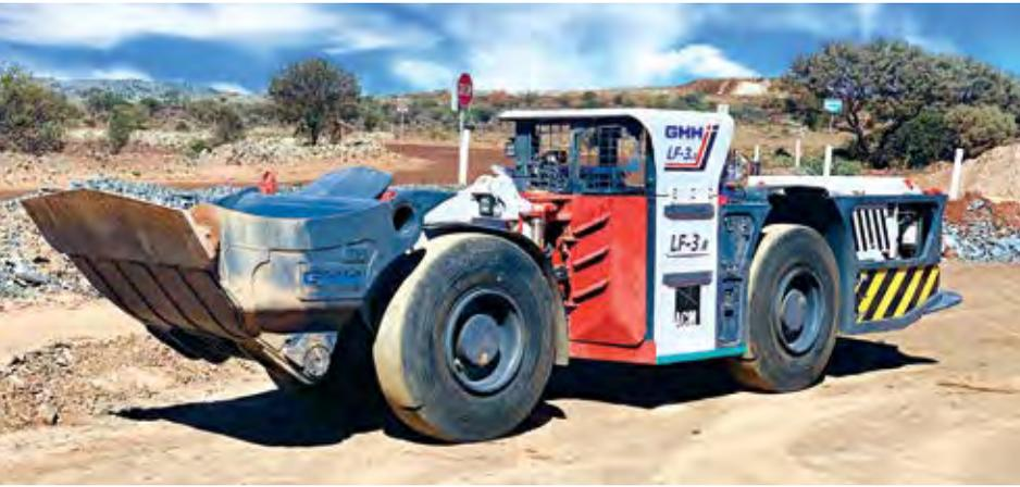
The LF-3 has an operating weight of 11 mt, a standard bucket capacity of 1.5 m<sup>3</sup>, and a payload capacity of 3.5 mt. (Photo: GHH)
