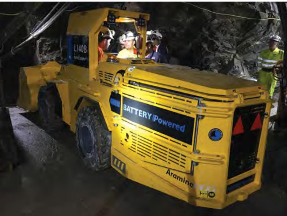
With a 0.7-m<sup>3</sup> bucket, the battery-powered L140B has a tramping capacity of 1,300 kg, tilt breakout force of 32 kN and lift breakout force of 35 kN. (Photo: Aramine)
