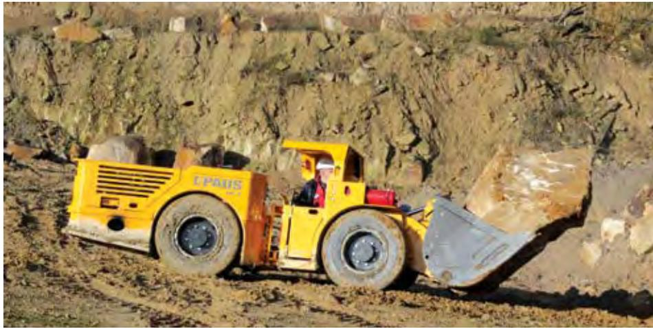
The PFL 8 LHD has a 0.8 m<sup>3</sup> bucket, a payload capacity of 1.5 mt, breakout force of up to 40 kN, an operating weight of 6.3 mt, and engine power of 69 kW. (Photo: Paus)
